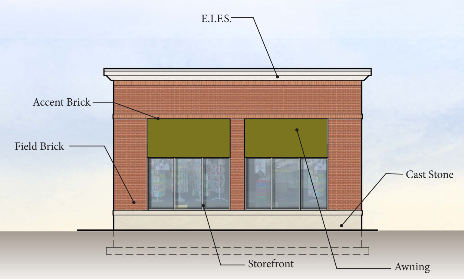
5 SOUTH WEST ELEVATION 1/8"=1'-0"
