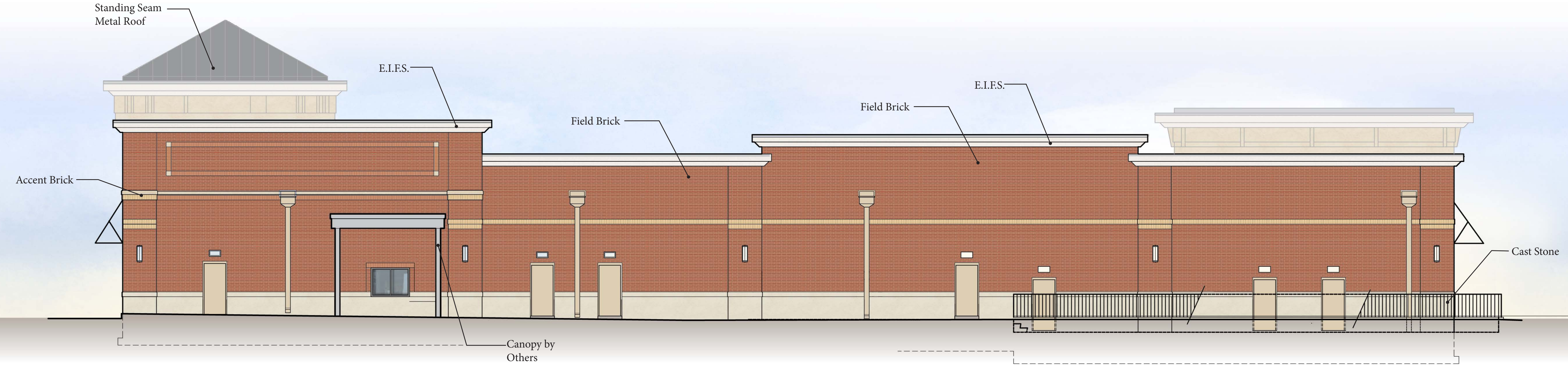
2 NORTH ELEVATION (REAR) 1/8"=1'-0"
